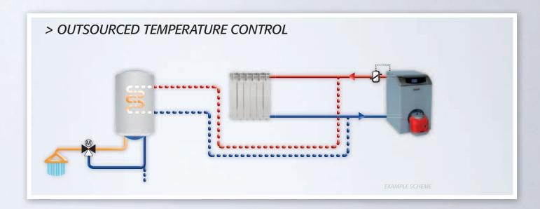
Ferroli indirect combi water heater is available also with a probe pocket on the top of the tank. As a consequence temperature will be independent from the auxiliary heating.
